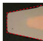
Weller WSW after 10,000 solder cycles
