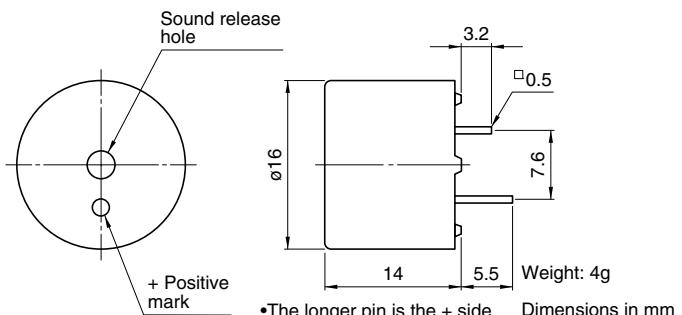
**SD1614TT-B3M(Applicable to automobile) / ø16mm TYPE****FEATURES**
