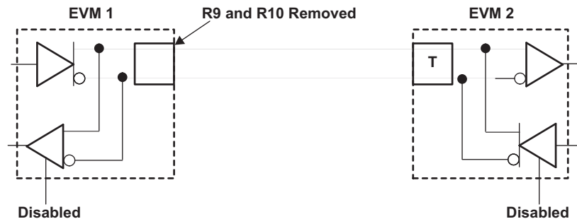
Figure 3. Point-to-Point Simplex Circuit
