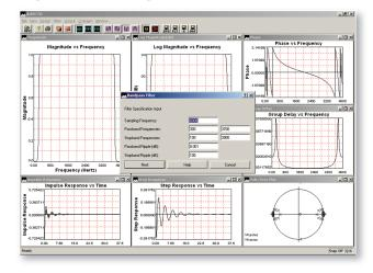
The Digital Filter Design Tool makes designing and analyzing FIR and IIR filters easy. When the user enters frequency specifications, the tool automatically generates the filter code and coefficients. Graphical output windows provide the desired filter's characteristics.
