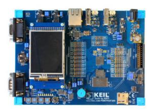
The Keil MCBSTM32F400 Evaluation Board enables you to create and test working programs based on the STMicroelectronics STM32 F4xx series of ARM Cortex™-M4 processor-based devices.
