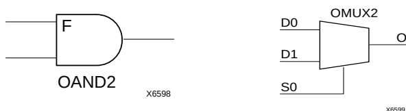
Figure 20: AND & MUX Symbols in XC4000X IOB
