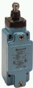
Global Limit Switches Series GLS: Top Roller Plunger, 1NC 1NO Slow Action Break-Before-Make (B.B.M.), PG13.5
