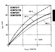
Figure 6: Typical loig vs.  $V^+$  - Vout,  $4.5V \le V^+ \le 6.0V$
