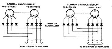
Figure 12: Thumbwheel switch/diode connections
