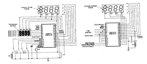
Figure 1: Test Circuits, showing the ICM7217 in the Common-Anode Version and the ICM7227 in the Common-Cathode Version
