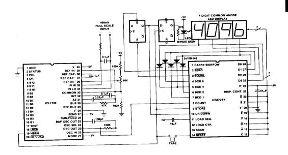
Figure 24: Auto-Tare System for A/D Converter
