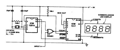
Figure 23: Precision Frequency Counter (~1MHz Maximum)
