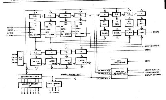
Figure 2: ICM7217 Functional Block Diagram
