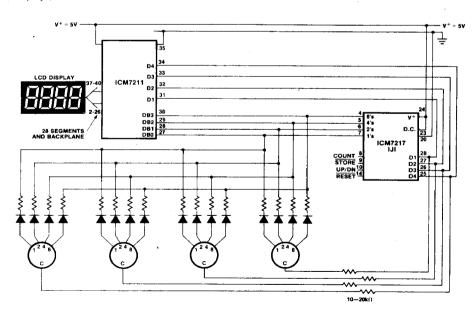
Figure 16: LCD Display Interface (with Thumbwheel Switches)
