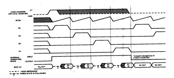
Figure 11: ICM7217 BCD I/O and LOADING TIMING
