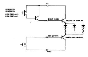
Figure 15: Driving High Current Displays
