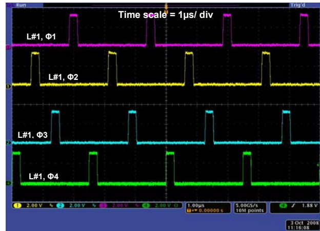
Figure 20: 4 phase PWM interleaved operation
