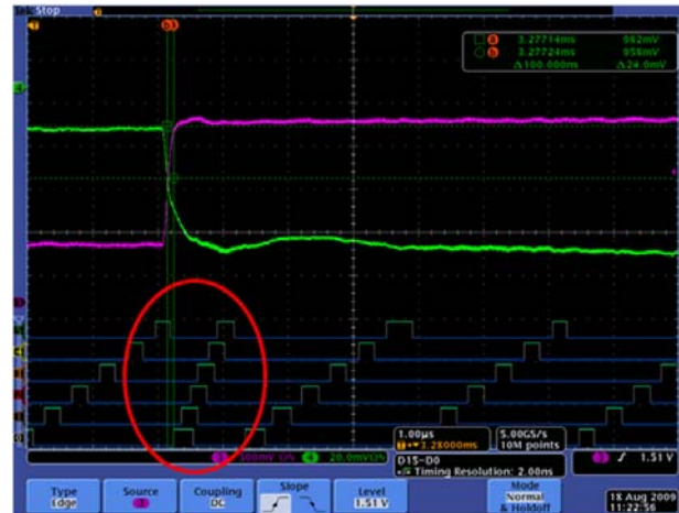
Figure 33: Load step with ATA enabled (L=215nH, Fsw=400kHz)
