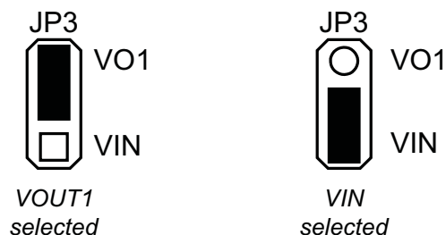
Figure 3. VINLR1 Jumper Setting
