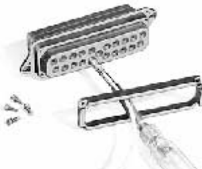
Inserting Coaxial & #12 Contacts
