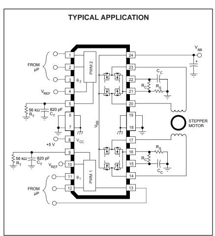
quence. This is accomplished by digitally selecting 100% drive current when only one phase is on and 67% drive current when two phases are on. Logic highs on both  $I_0$  and  $I_1$  turn-off all drivers to allow rapid current decay when switching phases. This helps to ensure proper motor operation at high step rates.
