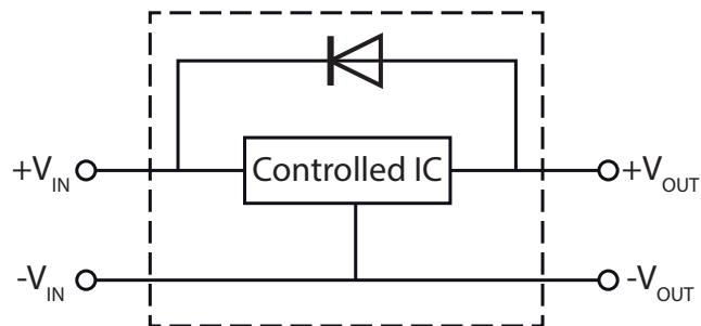
An internal blocking diode can prevent reverse current flow backwards into the output, as this can damage the converter when it is powered down.
