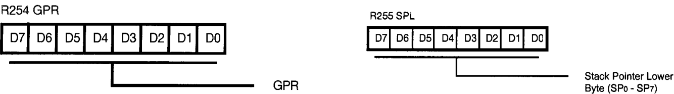
Figure 36. General Purpose Register (FEH: Read/Write) Figure 37. Stack Pointer Register (FFH: Read/Write)
