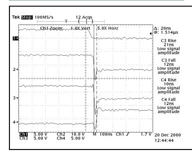
Figure 3: PWM input and Gate drive and phase node switching waveforms with time scale expanded. The MOSFETs driven are FDB7030BL . See Figure 4 (Evaluation Board Schematic)
