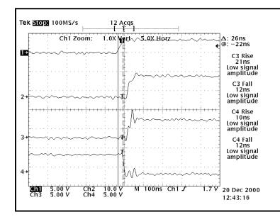
Figure 2: PWM input and Gate drive and phase node switching waveforms with time scale expanded. The MOSFETs driven are FDB7030BL . See Figure 4 (Evaluation
