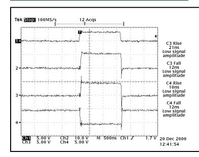
Figure 1: PWM input and Gate drive switching waveforms. The MOSFETs driven are FDB7030BL. See Figure 4 (Evaluation Board Schematic)
