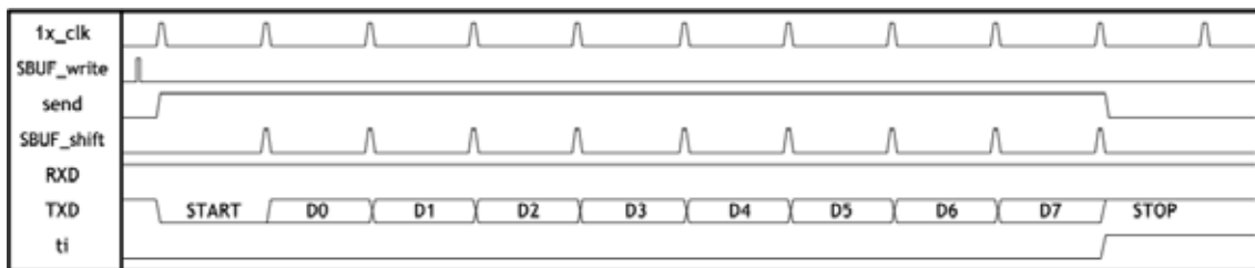
Figure 6.8 Timing Diagram for UART Transmission Mode1
