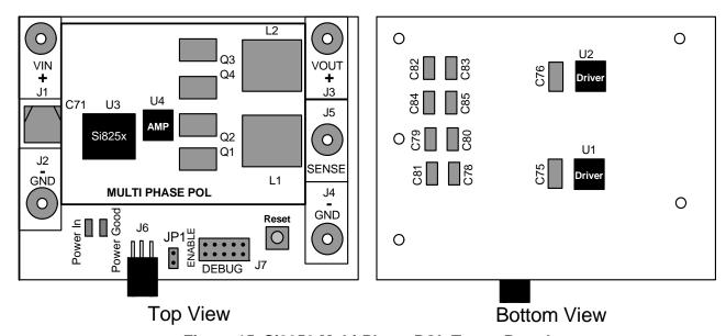
Figure 15. Si8250 Multi-Phase POL Target Board
