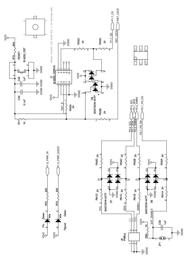
Figure 19. Si8250 Multi-Phase POL Target Board Schematic (Debug)
