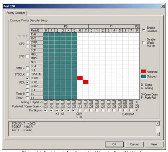
Figure 14. Peripheral Configuration Wizard—Port I/O Window
