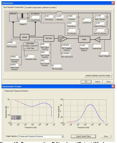
Figure 12. Compensation Editor, Input/Output Windows
