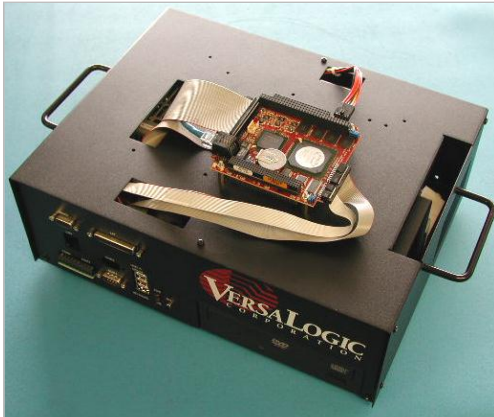
Figure 9. Example PC/104 Board Installation
