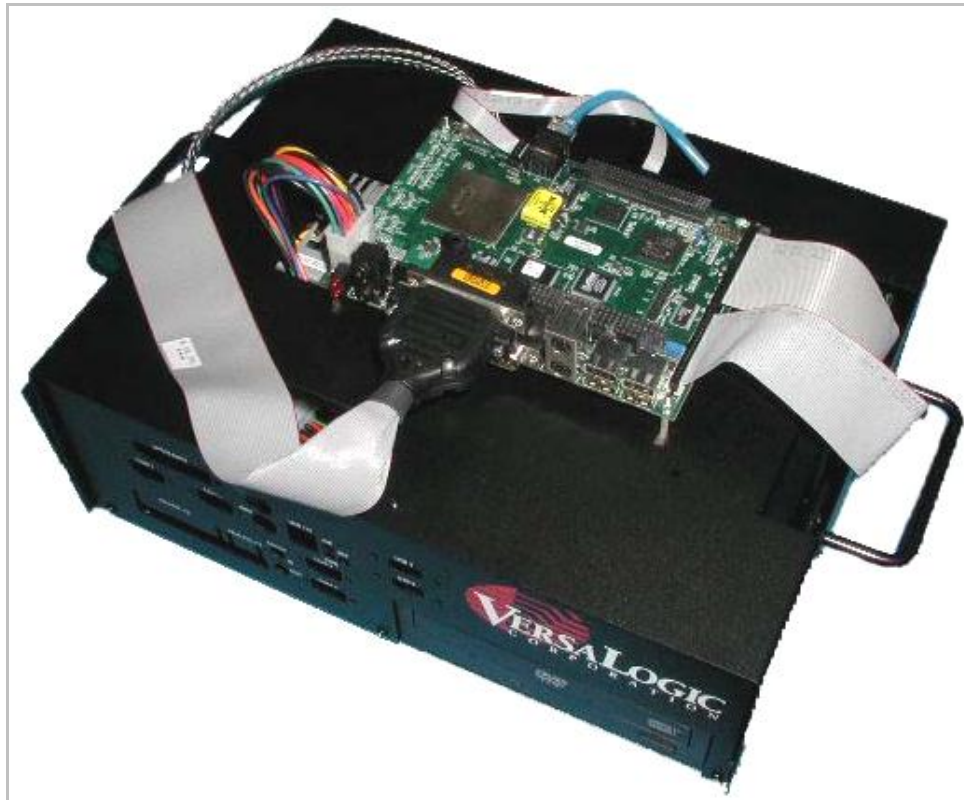
Figure 11. Example EPIC Board Installation
