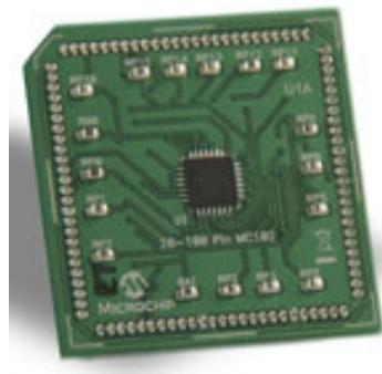
This PIM comes with a 28-pin dsPIC33FJ16MC102 QFN device. It is intended to be used to control the Microchip MCHV (DM330023), MCLV (DM330021) or MCSM (DM330022) motor control development boards. Notice: use of this PIN with the MCHV development board DM330023 Revision 4 or earlier (see product label), must be upgraded to support this PIM. Please contact the local Microchip sales office to obtain this free upgrade.
