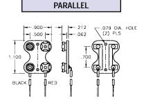
Contacts: Steel, Nickel Plate Wire: #22 AWG, 7/30 Prebond End Strip: .375 Long, Tinned
