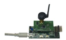
Plug the CC2530EM into the target board EM connector and connect the antenna
