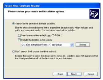
After the driver is installed the target module will be assigned a COM port. To see the COM port number, open the Windows Control panel – System – Hardware – Device Manager and check the COM port number under Ports (COM and LPT). The target board will be listed as a **TUSB3410 Device**, (COM69 in this example)
