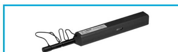
Insert the one-click cleaner into the insulator and push until an audible "click" is heard. The cleaner uses a mechanical push action to advance an optical grade cleaning tape. More than 500 cleaning per cleaner. Product includes special LEMO F2 ferrule adaptor.
