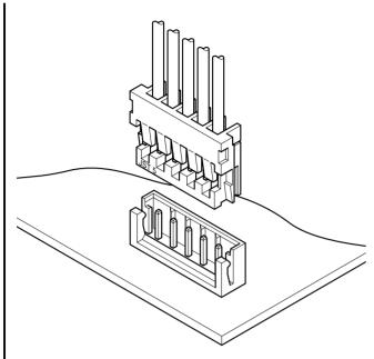
This 2.5mm pitch connector for printed circuit boards has a thin construction. The in-line method provides high-density capability to the end user.
