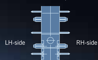
Side definition with terminals and location pins
