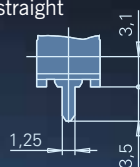
PCB terminal 1,3x0,5 mm straight
