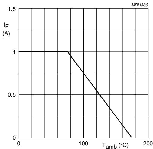
Fig.2 Maximum forward current as a function of ambient temperature.
