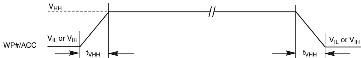
Figure 18. Accelerated Program Timing Diagram
