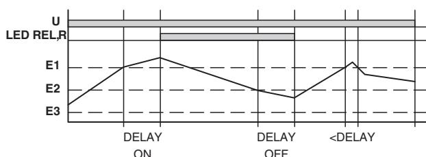
Connection of probe rods E1, E2, and E3. Probe rod E3 does not have to be connected if the container wall is made of metal.
