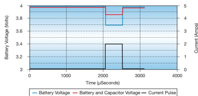
Figure 5. GSM Pulse
