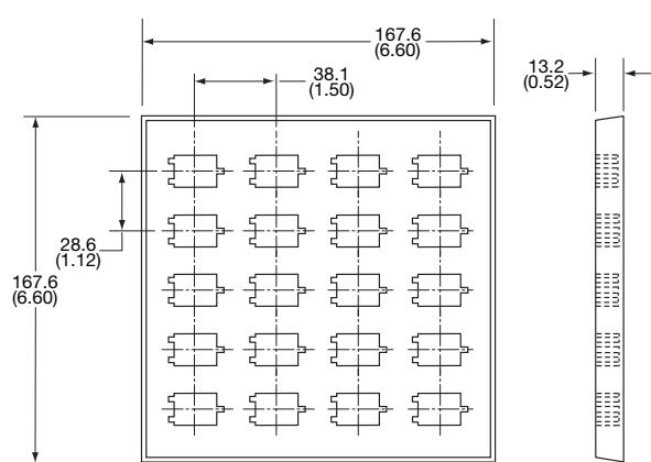
This specification applies when our electrochemical supercapacitors are packed using a 165mm by 165mm container. The parts are held in place by a 166mm by 166mm lid.
