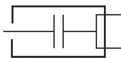
Common terminals connected to case
