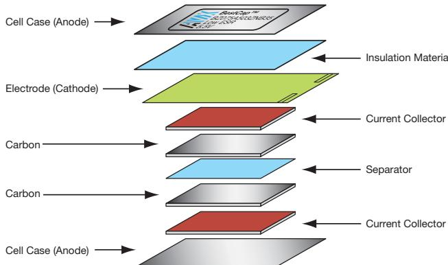
Electrons are relatively fast moving and therefore transfer charge "instantly." However, ions have to move relatively slowly from anode to cathode, and hence a finite time is needed to establish the full nominal capacitance of the device. This nominal capacitance is normally measured at 1 second.
