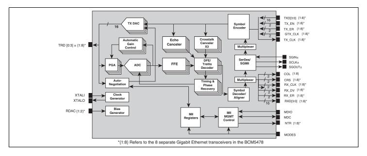
The BCM5478 consists of eight complete 10/100/1000BASE-T Gigabit Ethernet transceivers integrated on a single monolithic CMOS chip. The BCM5478 is optimized for low power and small footprint size to enable high-port-density applications. The BCM5478 enables a new class of cost-effective Gigabit Ethernet equipment by lowering system cost and reducing power dissipation by nearly 30 percent, driving the delivery of Gigabit Ethernet bandwidth to the desktop.
