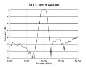
SFELG10M7 series for FM-receivers are monolithic type ceramic filters which use the thickness expander mode of the piezoelectric ceramic.
