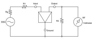
Rg+R1 =R2 : Input/Output Impedance
