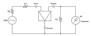
Rg+R1 =R2 : Input/Output Impedance
