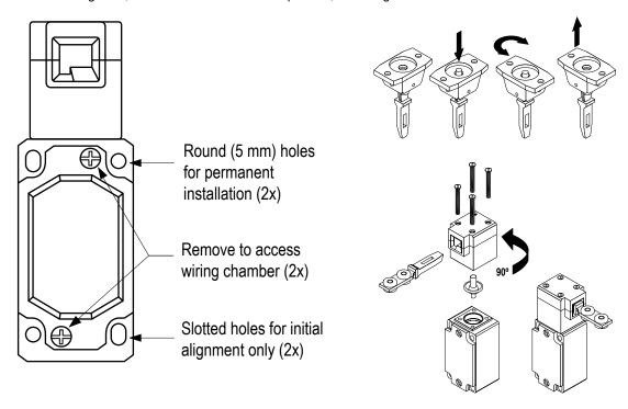
The mounting holes in the switch body accept M5 (#10) screws. There are four holes on a standard limit switch mounting pattern of  $30 \times 60$  millimeters. The two mounting holes on the actuator are spaced 20 millimeters apart. The grommet and sleeve design allows a small amount of movement (i.e., misalignment) when the actuator engages the switch body. The sleeves accept M4.5 (#8) screws.
