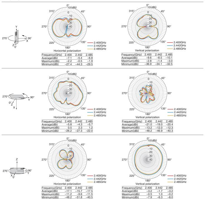
• Tested antenna has been soldered. Evaluation board size is 120×65×1 mm.
