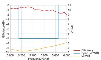
$\bullet$  Tested antenna has been soldered. Evaluation board size is 120x65x1 mm.
