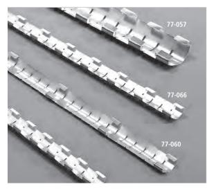
Laird Technologies introduces Variable Slot Mount shielding, which eliminates the use of long slots while still utilizing the easy installation method of slot mount shielding. Fingers are removed from the strip in areas where a mounting slot is not present. The Variable Slot Mount shielding strips can be customized to any patterned series of slots.
