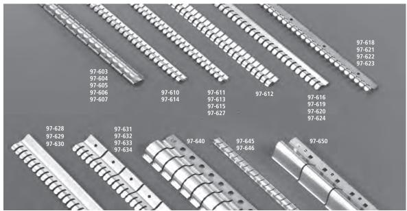
This series from Laird Technologies is designed for use where high temperature or other design considerations preclude the use of adhesive-mounted gasketing. Yet it provides the same shielding characteristics and effectiveness as on Sticky Fingers® mounted series. Clip-On Gaskets offer shielding effectiveness >100 dB for 100 MHz plane wave. All are available in your choice of finishes, see page 17.
