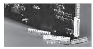
This product offers a clip-on design that permits shielding to a perpendicular surface.
