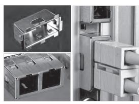
Laird Technologies provides fiber optic shielding, which provides excellent EMI shielding around the faceplate aperture which houses board mounted fiber optic transceivers. This EMI shield easily fits over the industry standard 1 x 9 style fiber optic transceiver with a duplex SC connector. The shielded transceiver is then inserted into the faceplate.
