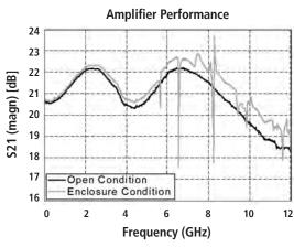
Figure 2. Performance of Amplifier in Open Condition and Inside Enclosure
