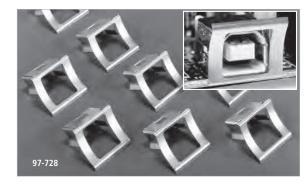
Laird Technologies offers the USB (Universal Serial Bus) Type B connector gasket. The unique design easily snaps onto the connector prior to placement on the printed circuit board and fits all Series B USB right angle connector brands. Made from high performance beryllium copper, these gaskets provide superior grounding characteristics and enhances the shielding of the connector due to the short electrical path to the ground plane provided when the gasket makes contact with the connector.
