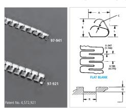
Series 97-941/921 are low compression, flexible beryllium copper contact strips for applications where a continuous shield must conform to irregular shapes and turn tight radius corners in either direction.
