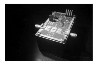
Figure 1. Variable Gain Broadband Amplifier 100 MHz to 12 GHz
