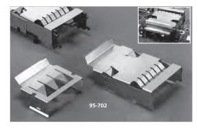
Laird Technologies offers the GBIC Shield for reducing emissions from GBIC (GigaBit Interface Converter) fiber optic transceivers. Fiber optic transceivers can be a troublesome source of EMI because they emit high-frequency signals and are located adjacent to large apertures in the enclosure. The GBIC Fiber Optic Shield assembly reduces the radiated emissions from the transceivers by conducting interference current away from the transceiver and onto the
