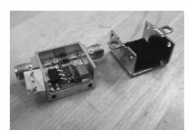
Figure 5. Amplifier and Enclosure with Lossy Foam Inside
