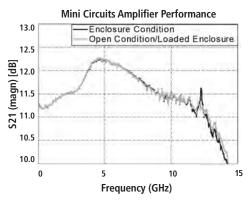
Figure 6. Performance in Enclosure and Using Foam Absorber
