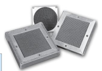
Vent panels range from 3 in. (76,2 mm) to 18 in. (457,2 mm) square in standard sizes, and can be ordered with either 0.50 in. (12,7 mm) thick or space-saving 0.25 in. (6,4 mm) thick honeycombs.
