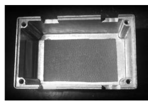
Figure 3. Enclosure with Q-Zorb PN 2238 Installed
