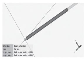
Figure 7. Microwave CST Model of Cable with Q-Zorb Coating
