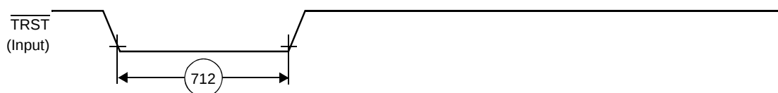
Figure 25. \overline{\text{TRST}} Timing Diagram
