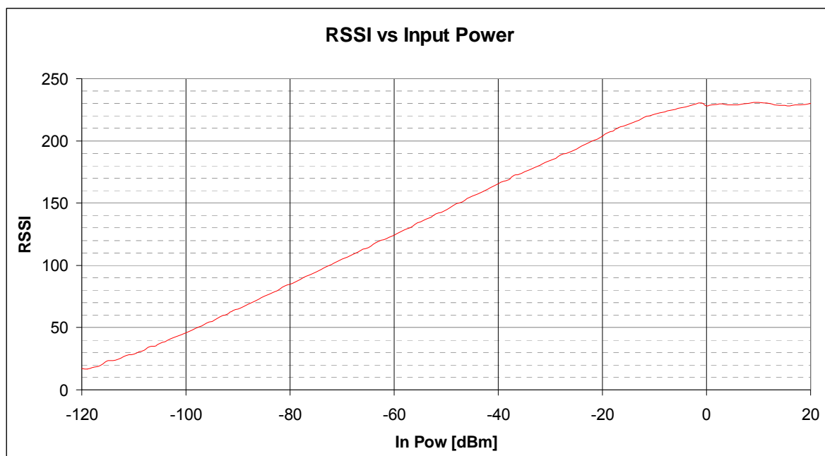
Figure 23.25. RSSI Value vs. Input Power
