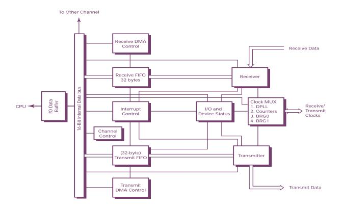
Interrupts are supported with a daisy-chain hierarchy, with the two channels having completely separate interrupt structures.
