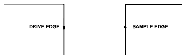
Figure 25. SPI Mode 3 SCLK Edges
