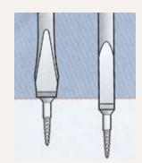
perfectly. Slotted screwdrivers are made with flared tips and parallel tips. For most work select a flared tip screwdriver, but you should select a parallel tip that is the same width as the screw slot, if you need to drive the screw below the surface of the wood without damage. Select a tip that matches the width of the screw slot, too wide and it will damage the work, too narrow and it may damage the screw slot.
