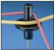
In the "up" position to form harness.
