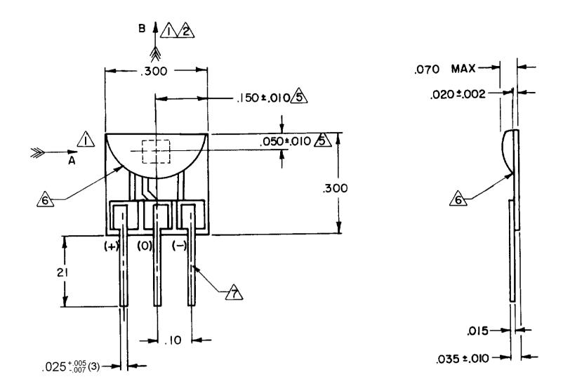
TO TEST THE SWITCH AGAINST THE SPECIFIED OPERATING CHARACTERISTICS THE SWITCH MUST BE PLACED IN A HELMHOLTZ COIL FIELD AND GIVEN THE FOLLOWING HISTORY: 35 GAUSS MINIMUM IN DIRECTION "A": 35 GAUSS MINIMUM IN DIRECTION "B", TEST TO THE OPERATING CHARACTERISTICS IN DIRECTION "B" (TFIS ASSUMES THE CONVENTION THAT THE DIRECTION OF THE EXTERNAL FLUX OF A MAGNET IS FROM THE NORTH TO THE SOUTH POLE OF A MAGNET)
