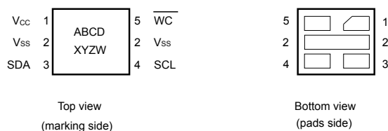
Figure 3. UFDFPN5 (DFN5) package connections
