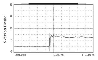
ESD Test Pulse - 25 kilovolt, 1/30 ns (waveshape)
