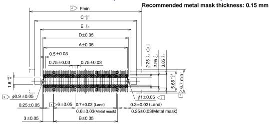
Note 1 Cross-hatched portions, totaling n places, indicate the ground circuits.
