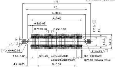
Note  $\square$  Cross-hatched portions, totaling n places, indicate the ground circuits.
