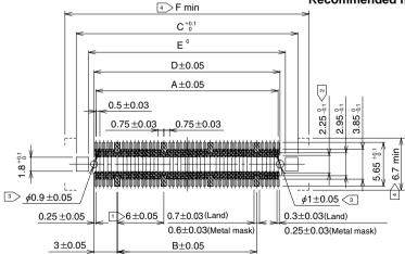
Note 1 Cross-hatched portions, totaling n places, indicate the ground circuits.
