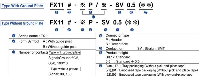
Note 2: Information contained in this catalog represents general requirements for this Series. Contact us for the drawings and specifications for a specific part number shown.
