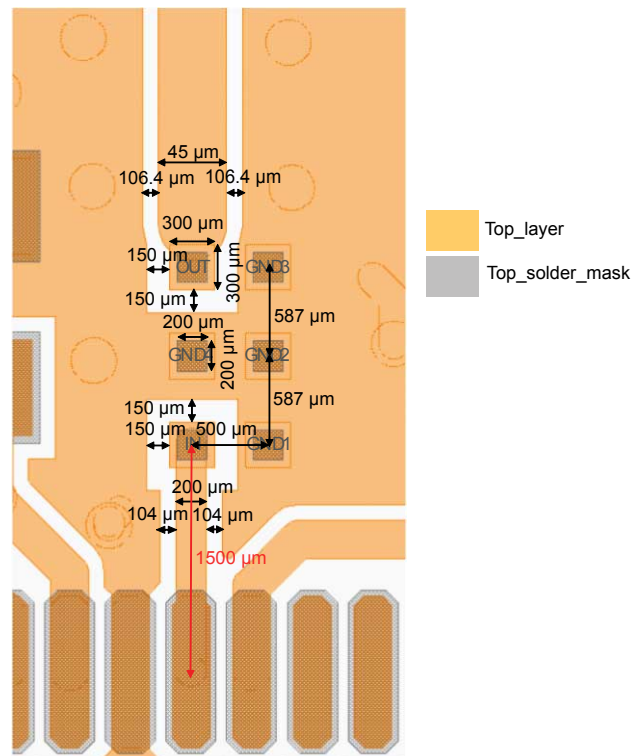
Figure 13. PCB land pattern recommendations
