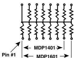
13 and 15 resistors with one pin common
