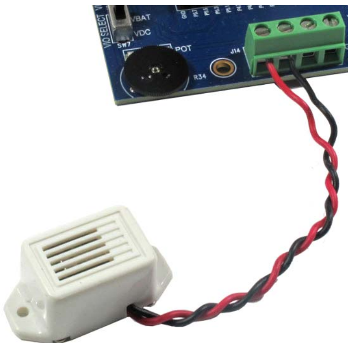
Figure 26. Optional 3 V Buzzer
