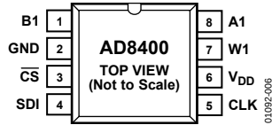
Figure 6. AD8400 Pin Configuration
