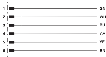
Contact assignment of 7/8" plug
