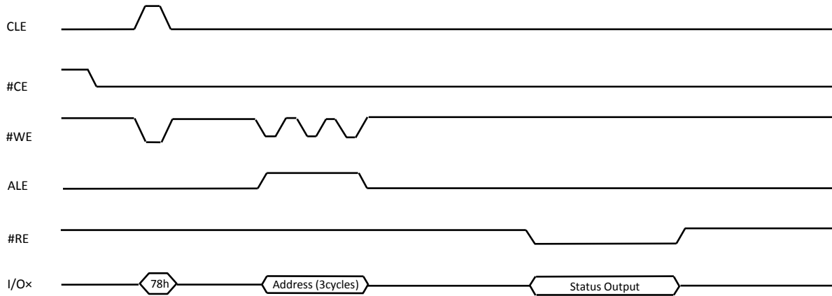
Figure 9-8 Read Status Enhanced (78h) Operation
