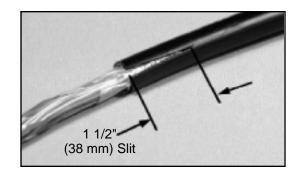
3.03 Make a 1" (25 mm) slit in the outer sheath and shield. Lift corners for base insertion.
