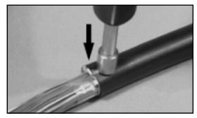
4.04 Attach bond assembly over stud and tighten firmly with securing nut.
