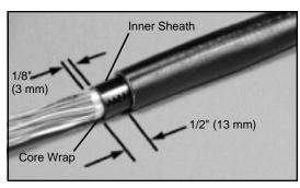
Note: On cables less than 3/4" (19 mm) in diameter, cut a 1 1/2" (38 mm) slit in the sheath opposite connector location. Then complete procedure.
