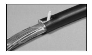
4.03 Place terminal wrench over stud and push down to bend corners and pull slit together.
